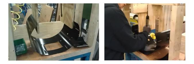
To reduce the level of MSD risk, the assembly process was changed to install the access plate prior to riveting the can together. A fixture was fabricated to hold the can open while the access plate is being installed. A straight or "in-line" pneumatic screwdriver (on a tool balancer) is now used to improve upper extremity work postures and eliminate the force required.
