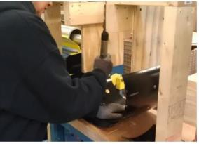
To reduce the level of MSD risk, the assembly process was changed to install the access plate prior to riveting the can together. A fixture was fabricated to hold the can open while the access plate is being installed. A straight or "in-line" pneumatic screwdriver (on a tool balancer) is now used to improve upper extremity work postures and eliminate the force required.
