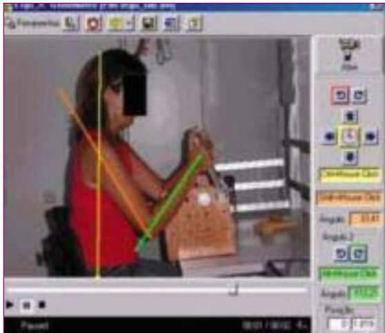
Figure 33. Use of ERGO_X Tools to analyse worker movements
